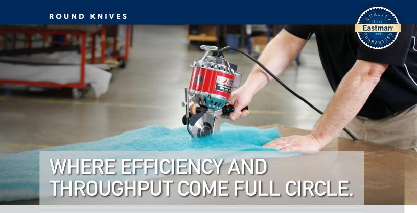
Commonly used to cut straight lines or large radius curves, Eastman round knives are a combination of versatility, power, and ease of use – all in one.
