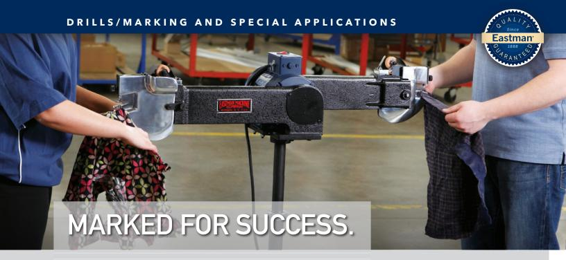
Eastman drills and marking machines work through numerous layers of material allowing for easy buttonhole, darts or other markings.
