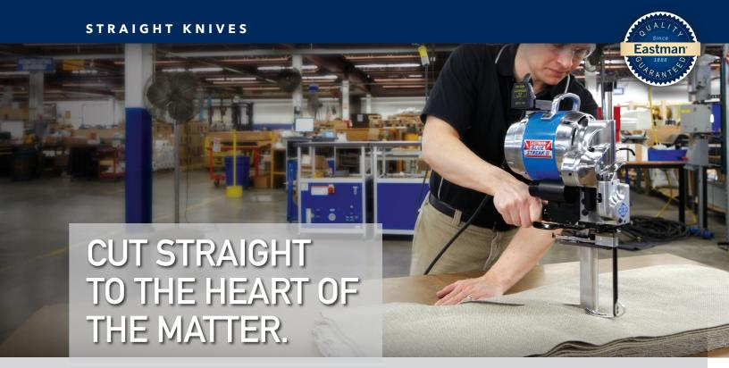
The industry standard since 1888, Eastman straight knife machines are engineered with high-speed reciprocating cutting technology to cut the most diverse range of traditional, modern and industrial fabrics in the market today.
