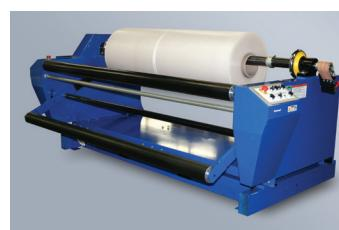
Introduce rolled fabrics to the cutting table in a relaxed or tensionless state with precise edge control. A full range of options in a variety of widths for numerous roll capacity specifications, Eastman manufactures in tandem with industry requirements to ensure streamlined, accurate and controlled material feeding enters the machine.
